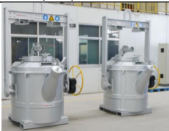
Figure 34: Molten aluminum can be shipped through specialized tea-pot shaped container
